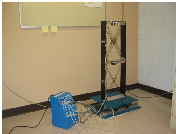
Fig. 6-1. The shaking table with the 2DOF shear building structure mounted on it
