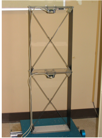
Fig. 6-4. Front view of the experimental 2DOF structure including the added weak steel springs
