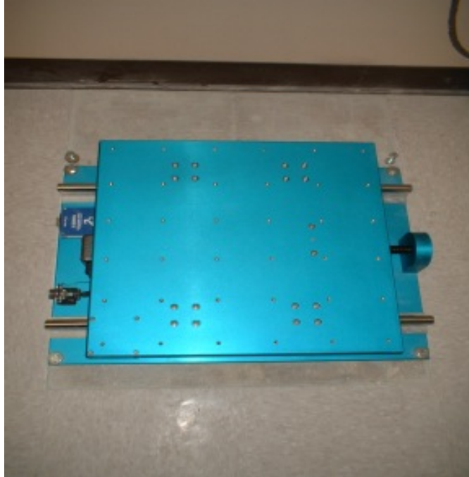
Fig. 6-2. Plan view of the shaking table
